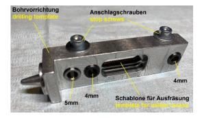
In the first step, the fastening holes for the lock housing must be drilled into the canopy frame.
