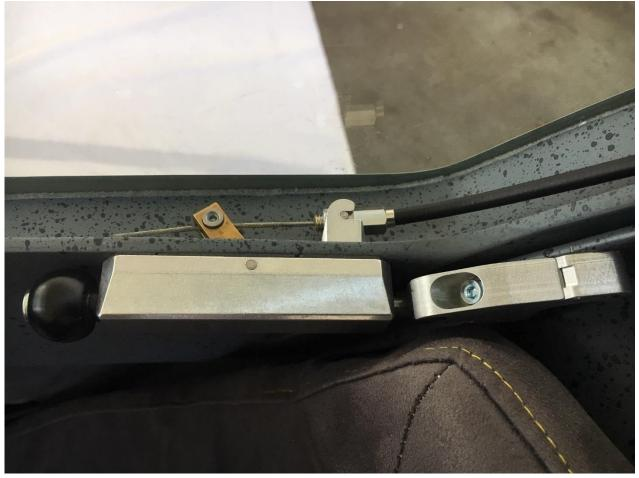
**Description:** The additional canopy lock prevents the canopy frame from bending open on both sides, which can occur due to strong suction at speeds of over 300 km / h.
